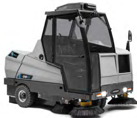
OBBL Direct load, front guide with Bullsystem® technology Cleaning path 1270/2100 mm
